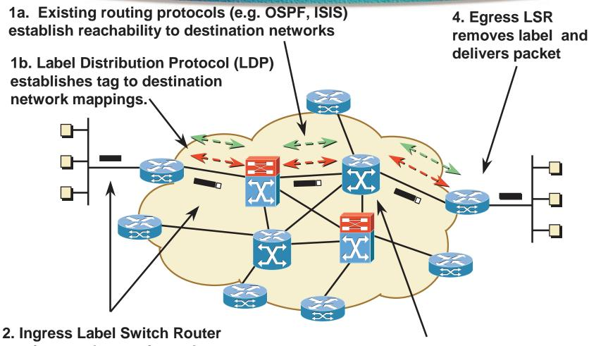
Ingress Label Switch Router receives packet, performs Layer
