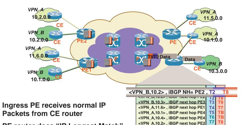
PE router does "IP Longest Match" from VPN\_B FIB, find iBGP next hop PE2 and *impose a stack of Labels's :* exterior Label T2 + Interior Label T8
