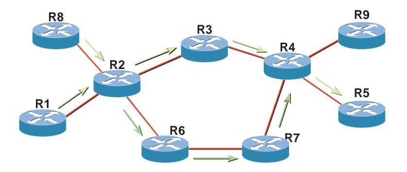
IP (Mostly) Uses Destination-Based Least-Cost Routing Flows from R8 and R1 Merge at R2 and Become Indistinguishab From R2, Traffic to R3, R4, R5, R9 Use Upper Route
