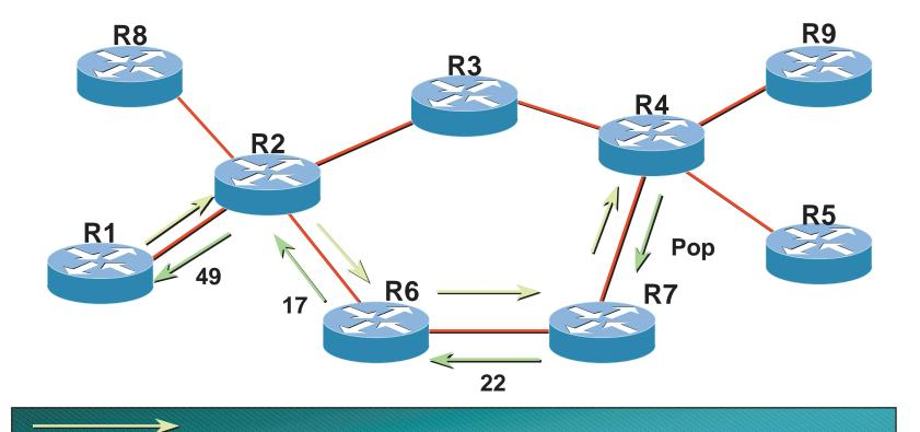
Setup: Carries Path (R1->R2->R6->R7->R4) and Tunnel ID
