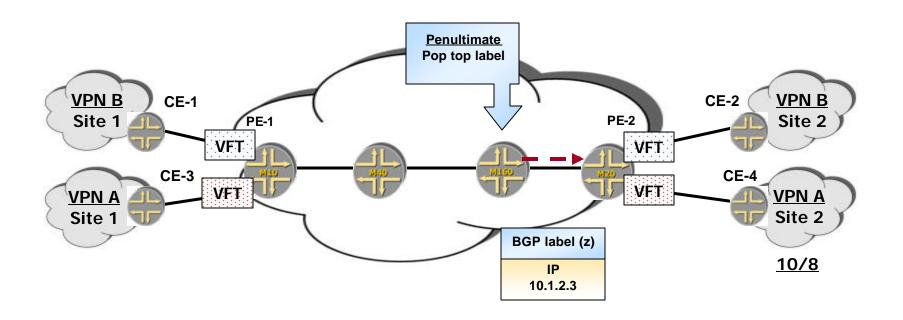
Penultimate hop popping (before reaching the egress PE router) removes the outer label
