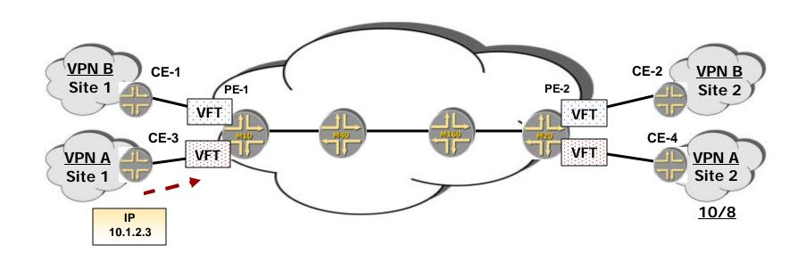
The CE device performs a traditional IPv4 lookup and sends packets to the PE router
