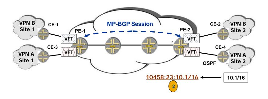
IPv4 address is added to the appropriate VRF
