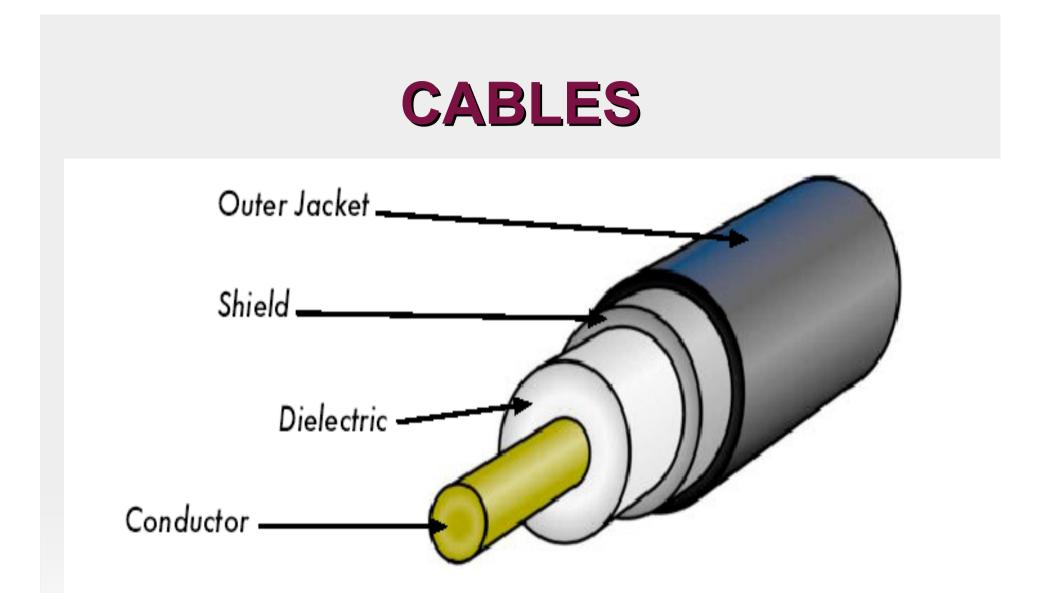
Coaxial cable with jacket, shield, dielectric, and core conductor e conductor.
