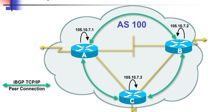
Loopback interfaces are normally used as the iBGP peer connection end-points
